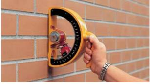
Pendulum hammer type PM to test mortar joints
