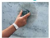
Smoothen test area with a grinding stone.
