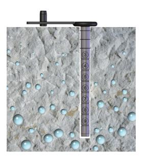
The moisture content inside the concrete is different to that on the surface. Surface based testing methods only measure up to 20 mm (%") at best and don't necessarily reflect reality. Therefore, the Hygropin uses the in-situ technology which identifies the actual moisture content inside the concrete.
