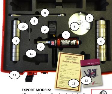
All export kits are fitted with a hydraulic tester body coupler, gauge couplers and an oil bottle with coupler.
