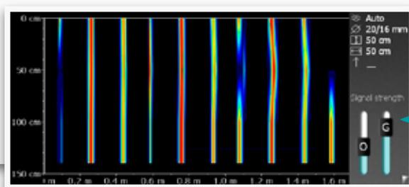
*By changing the Offset- and Gain-slider positions the signal strength range and resolution can be set and accordingly shown in a color spectrum, for example to display the first layer of rebars.*
