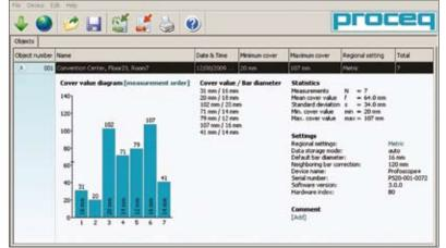
The graphic display of the Profoscope<sup>+</sup> shows all necessary information while acquiring data on site.
