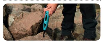
The world's most advanced rebound hammer, with unmatched dispersion characteristics, durability and measuring range has now been fully adapted for rock testing. The following features of the hammer make it ideal for rock testing applications:
